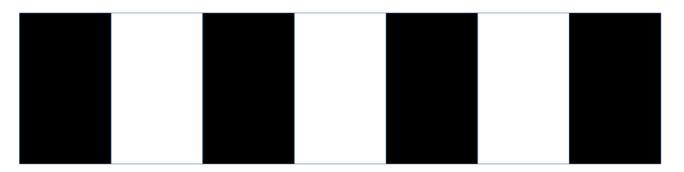
If the photocoupler is over the white area  $\rightarrow$  the right motor must run. If the photocoupler is over the black area  $\rightarrow$  the left motor must run.
