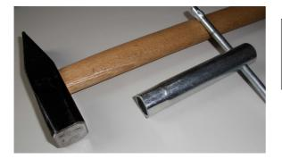
Tip: A hammer and a socket or small pipe are useful to press the ball bearing onto the axle.
