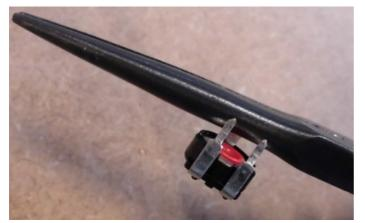
→ The "legs" of the adjustable resistor should be bent straight.
